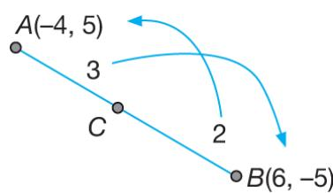
$$\begin{aligned} C &= \left( \frac{2(-4) + 3(6)}{3+2}, \frac{2(5) + 3(-5)}{3+2} \right) \\ &= (2, -1) \end{aligned}$$
